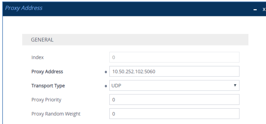
Figure 4-7: Configuring Proxy Address for SwyxWare IP-PBX
